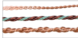
Copper wire twisted then hammered.
