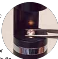
Determine whether diamonds have been fracture filled with this portable darkfield!
