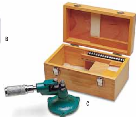
With a tap of a hammer, rings can be quickly and economically stretched. We recommend our rawhide mallets on page 102.
