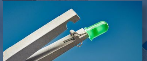
RX 601 forming pliers leave a standoff in wire and on LED leads.
