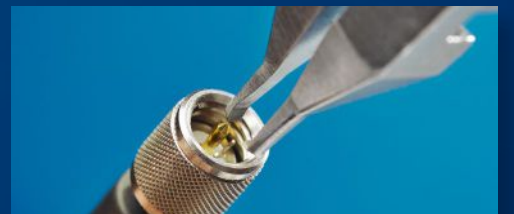
7292MI micro-mini end cutter is used to cut wire inside a mini connector.
